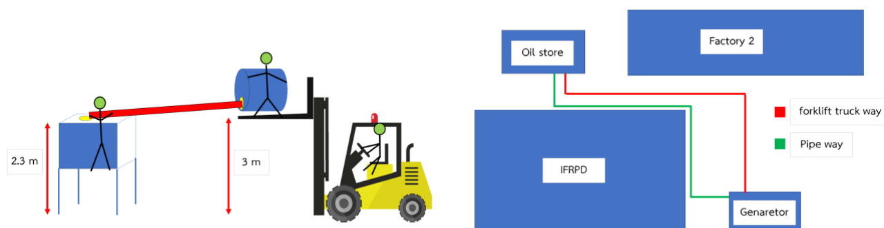
Figure 1. Graphic diagram illustrating (left) the current refill fuel method, which is inappropriate, causing a high risk of accidents occurring. (right) the top view of the semi-automatic piping system of fuel oil into power generator (green line) comparing the old system with forklift truck way (red line)
