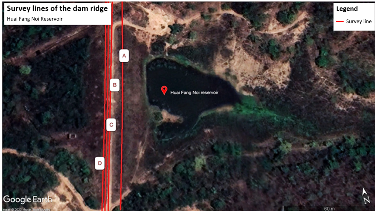
Figure 3. Electrical resistivity survey lines at Huai Fang Noi Reservoir, modified from Google Earth.
