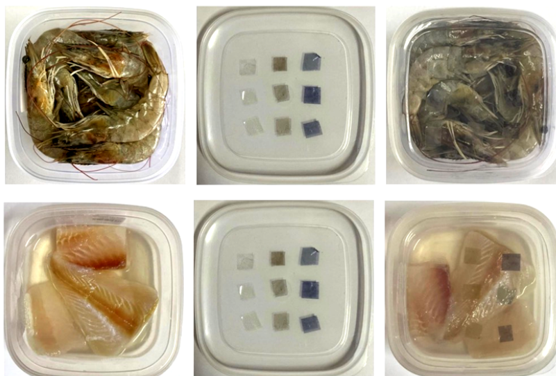
Figure 7. Intelligent film based on CMC/SA incorporated with JD mixed with BP applied for tracing sea food spoilage.
