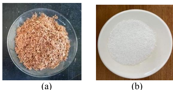
Figure 2. Untreated RH (a) and silica from rice husk after acid treatment and calcined at 900 °C (b).
