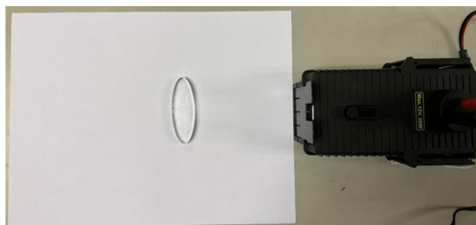
Figure 5. Experimental setup for light refraction through the DIY bifacial convex lens set.
